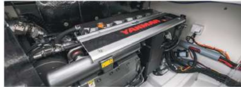
Yanmar 6LY - 440HK, with straight shaft.
